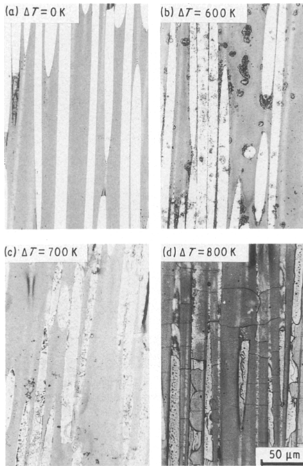
Figure 2 Typical optical micrographs of surface of the SiC fibre-reinforced borosilicate glass matrix composite (a) before and (b–d) after thermal shock at \Delta T 600 K, (c) 700 K and (d) 800 K.
